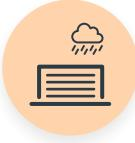
If film-faced formwork panels need to be stored temporarily outdoors, cover them with waterproof canvas. The panel edges should be protected from rain or ground water.
